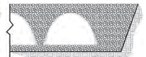
Perimeter Fully Backfilled
