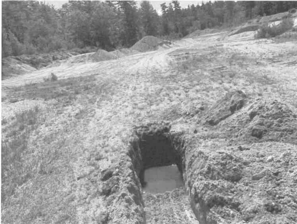
Photograph No. 11: View of Test Pit 12 showing Udipsamments soil with a wet substratum.
