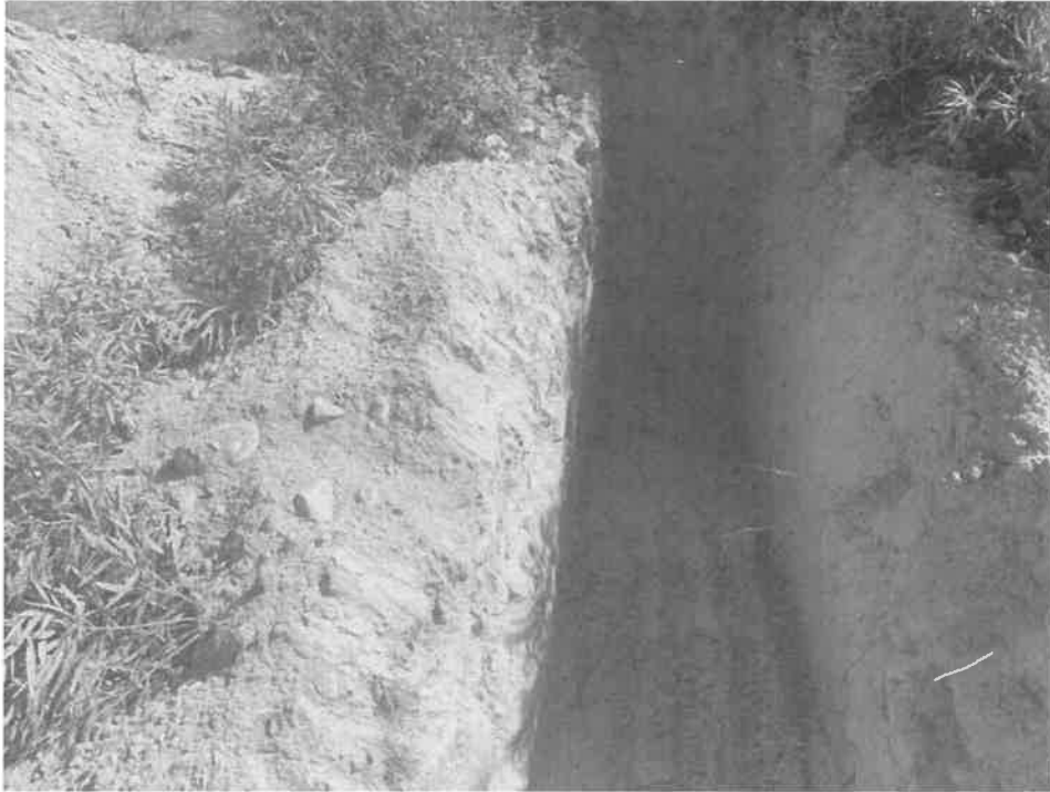
Photograph No. 7: View of Test Pit 4, showing Udipsamments soil with a wet substratum.
