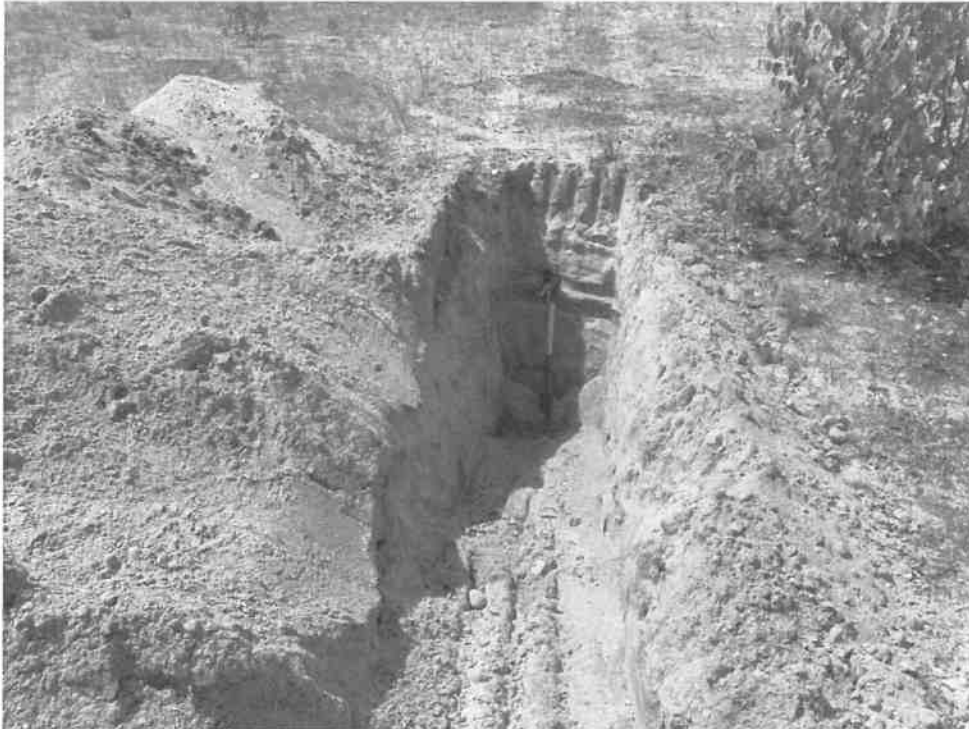
Photograph No. 15: View of Test Pit 20 showing Udipsamments soil with a wet substratum.
