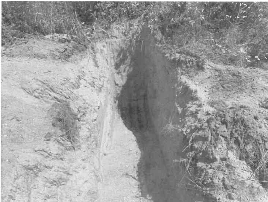
Photograph No. 10: View of Test Pit 11 showing Udipsamments soil with a wet substratum.
