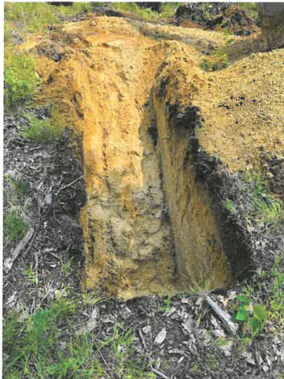
Photograph No. 4: View of sandy stratified drift aquifer deposits in Test Pit 19 in the northern portion of the Site to be developed. This area is mapped as Soil Unit 26 (Windsor).
