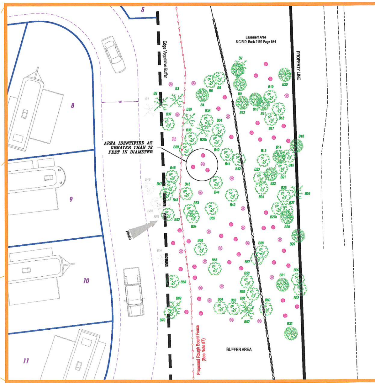
TYPICAL VEGETATION ENHANCEMENT SECTION Scale 1" = 10'
