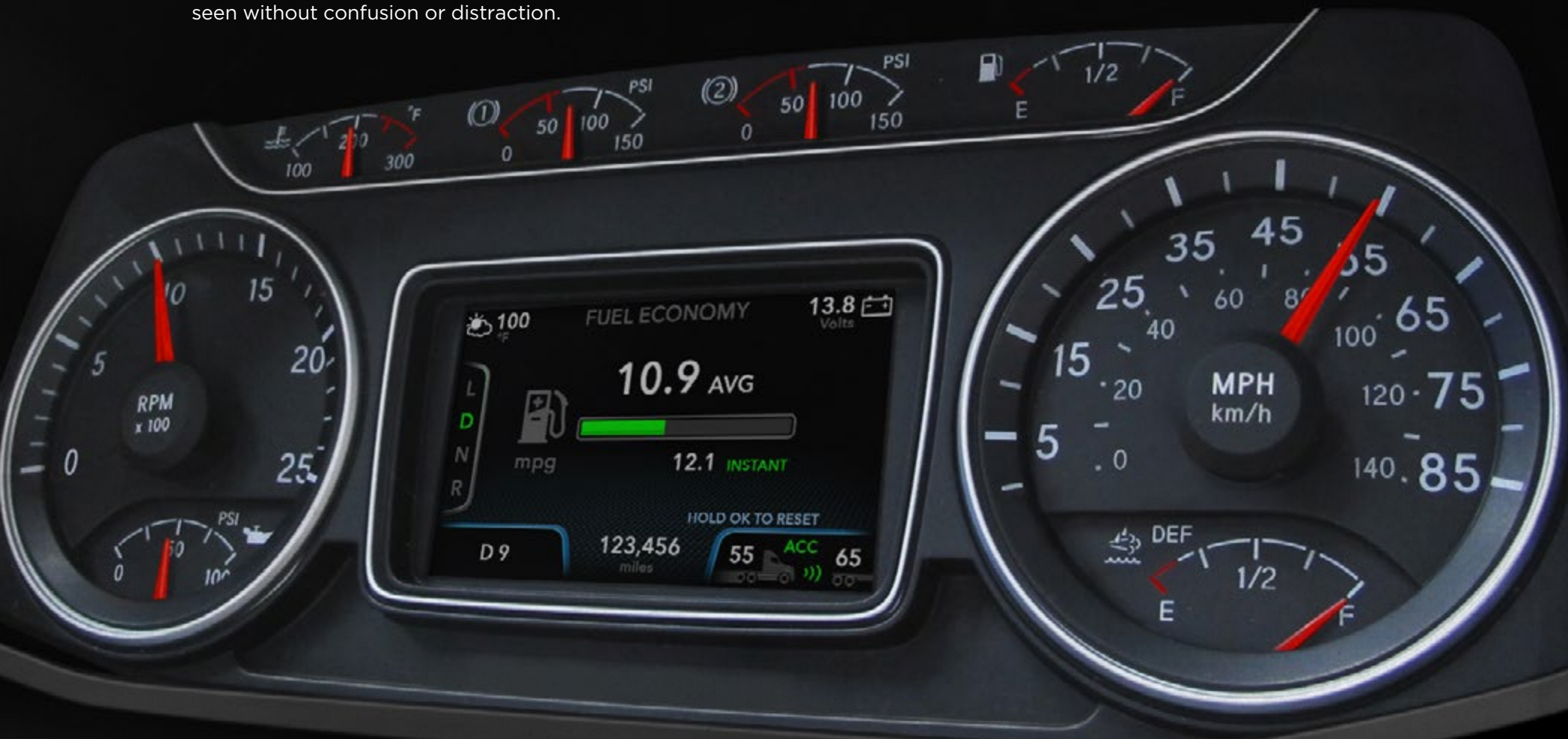
The color, illumination, legibility and even the type font and size of gauges is designed to deliver optimal viewing in varying light conditions, maximizing alertness and minimizing eye fatigue.
