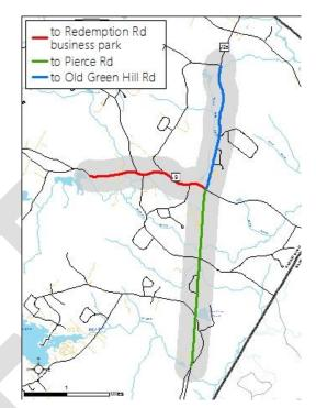
Figure 3: Possible water distribution lines and service area connecting the town center with current and potential business park locations.
